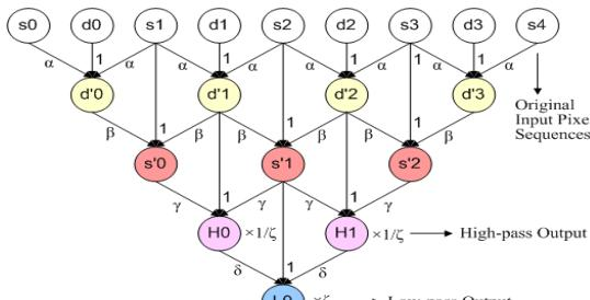
Fig. 1. The 9/7 LDWT structure.
